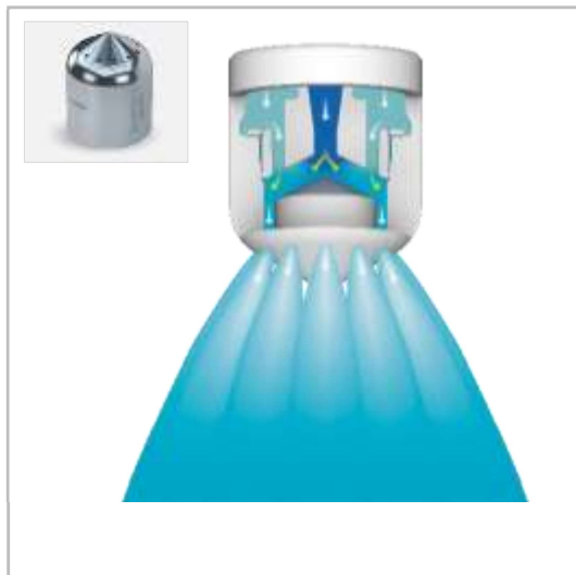
Illustration of the Lechler VarioJet nozzle
